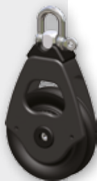
Art. 5400601 SWIVEL BLOCK Gewicht = 0.16kg 6mm Schäkel SWL = 800kg
