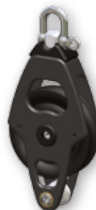
Art. 5400602 SWIVEL BLOCK Gewicht = 0.16kg 6mm Schäkel SWL = 800kg
