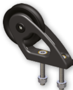
Art. 5400616 VERTICAL FIX Gewicht = 0.14kg Montage = 2x Ø6mm SWL = 800kg
