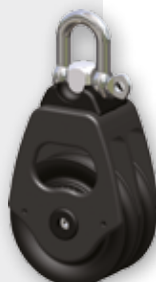
Art. 5400703 DOUBLE SHEAVE Gewicht = 0.38kg 8mm Schäkel SWL = 2200kg
