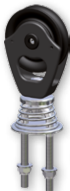
Art. 5400613 BLOCK U-BOLT Gewicht = 0.22kg Montage = 2x Ø6mm SWL = 800kg
