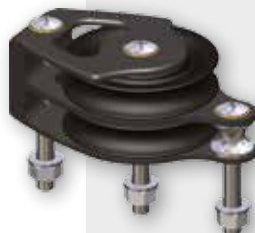
Art. 5400712 DOUBLE FOOT Gewicht = 0.26kg Montage = 3x Ø8mm SWL = 1300kg
