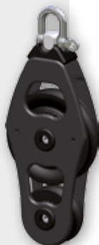
Art. 5400607 SINGLE FIDDLE Gewicht = 0.21kg 6mm Schäkel SWL = 800kg
