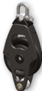
Art. 5400702 SWIVEL BLOCK Gewicht = 0.22kg 6mm Schäkel SWL = 1300kg
