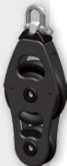
Art. 5400707 SINGLE FIDDLE Gewicht = 0.26kg 6mm Schäkel SWL = 1300kg
