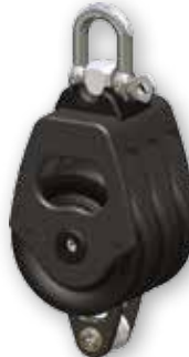
Art. 5400706 TRIPLE BECKET Gewicht = 0.52kg 8mm Schäkel SWL = 2200kg
