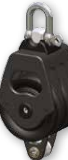
Art. 5400606 TRIPLE BECKET Gewicht = 0.43kg 8mm Schäkel SWL = 1300kg
