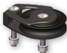
Art. 5400611 FOOT BLOCK Gewicht = 0.13kg Montage = 2x Ø6mm SWL = 800kg
