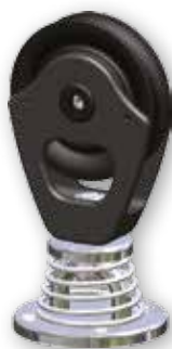
Art. 5400714 BLOCK PAD-EYE Gewicht = 0.41kg Montage = 4x Ø8mm SWL = 1300kg
