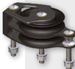
Art. 5400612 DOUBLE FOOT Gewicht = 0.22kg Montage = 3x Ø6mm SWL = 800kg
