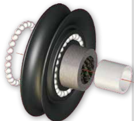
Art. 5400717 UP-DOWN Gewicht = 0.20kg Montage = 2x Ø8mm SWL = 1300kg
