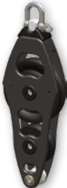
Art. 5400608 BECKET FIDDLE Gewicht = 0.23kg 6mm Schäkel SWL = 800kg
