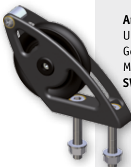
Art. 5400716 VERTICAL FIX Gewicht = 0.18kg Montage = 2x Ø8mm SWL = 1300kg
