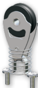
Art. 5400322 SADDLE BLOCK Gewicht = 46gr SWL = 400kg 2 x Ø5mm Schraube (inklusive)
