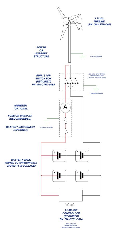
Fig-12: Simple 'Stand-Alone' battery-charging wiring diagram
