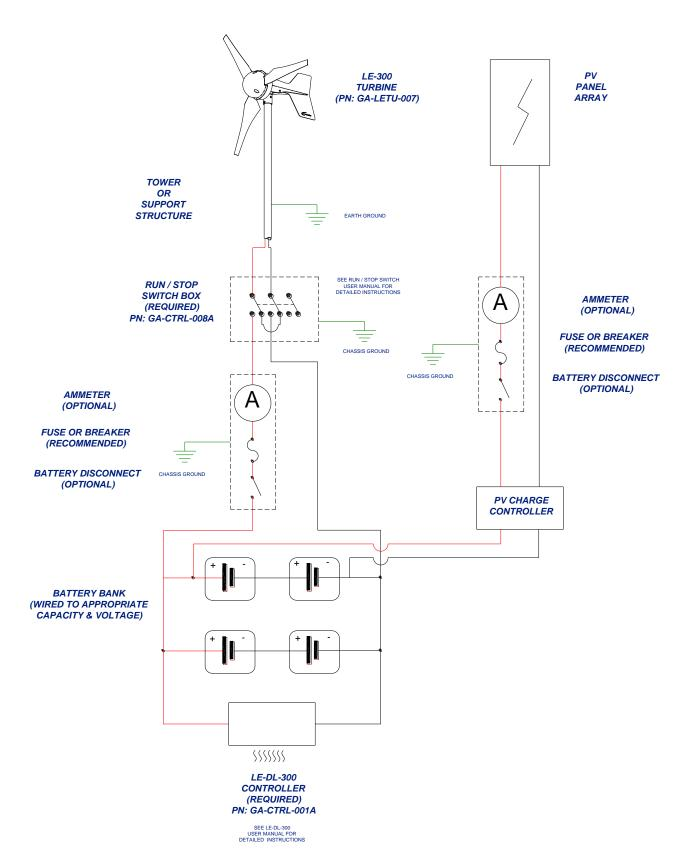
Fig-13: Typical 'Hybrid' wind /PV System wiring diagram
