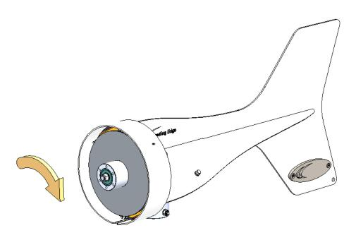
Fig-4: Checking magnet rotor rotation and coil-disc continuity
