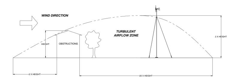
**Topography:** For areas of undulating ground, the turbine should be installed in the highest possible position avoiding wind barriers and turbulence. For areas that are generally flat, the turbine can be installed in any position. Remember that the LE300 has a low voltage output, so it is important to keep the cable run to the batteries / inverter as short as possible.
