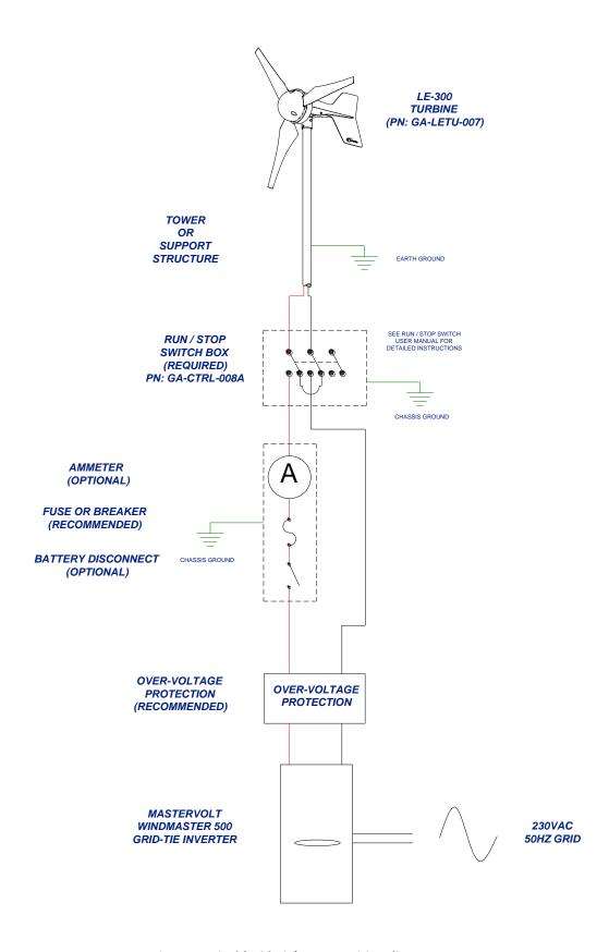
Fig-15: Typical 'Grid-Tie' system wiring diagram
